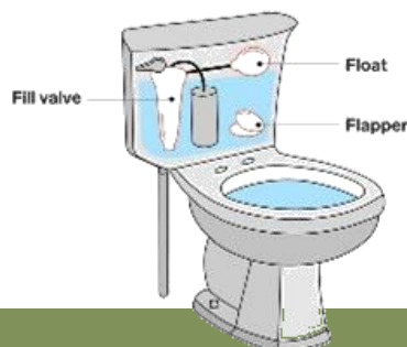
Common causes for a running toilet
